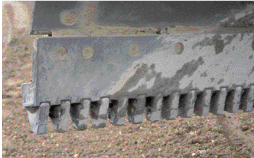
The carbide-tipped bits on a cutting edge can be a valuable tool in preparing a road for Chloride treatment. They penetrate the road and give a shallow scarifying effect to loosen and mix the existing gravel. This leaves a nice uniform loose layer of material on the surface.
